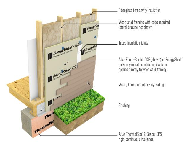
**Note:** Approved lateral bracing methods such as 1"×4" wood let-in-bracing, metal strap cross bracing, inset shear panels and structural sheathing at corners and at regular intervals must be used when polyiso foam is applied directly to wood stud framing. Consult architect, engineer, local code and code official for most appropriate solution.
